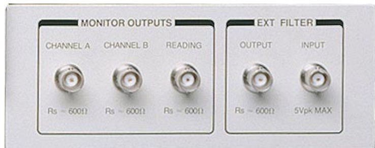
Figure 1-4 Monitor Outputs and External Filter Connections (Lower Right) Connector Panel
