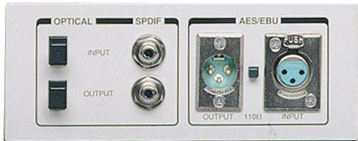
Figure 1-5 Digital Input/Output (Lower Left) Connector Panel
